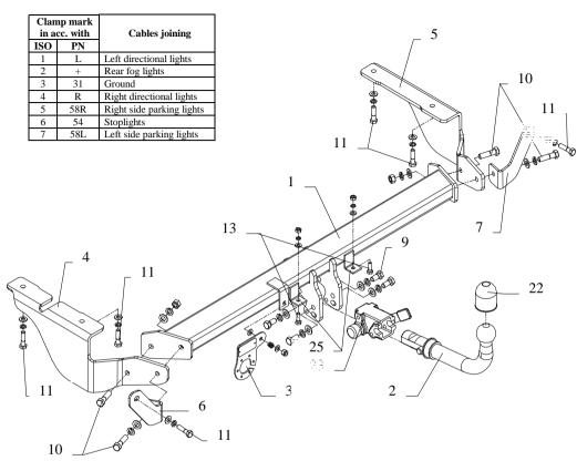
This towbar is designed to assembly in following cars: CITROEN C5 II ESTATE, produced since 10.2004 till 03.2008, catalogue no. P30A and is prepared to tow trailers max total weight 1600 kg and max vertical load 85 kg.
